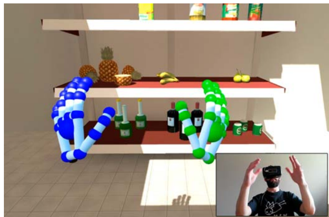
Figure 2: The second iteration of the VFS using the Oculus Rift DK2 and the Leap Motion technology to facilitate interaction with a virtual supermarket-shelf.
